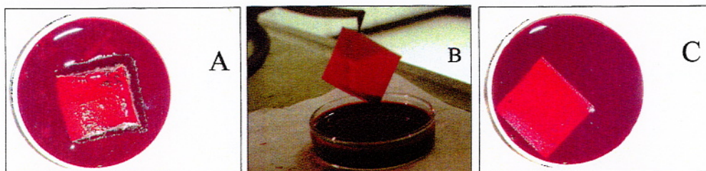
Figure 1. Visual inspection of the hemostatic pads in blood after an incubation time of 2 minutes. Type A pad (left) visible clots can be seen at the edge of the pads; type B pad (center) — pad sinks into blood, no visible clots were found on the pad; type C pad (right) — pad floats in blood, no visible clots were found on the pad.
